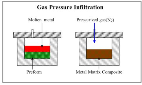
Gas Pressure Infiltration method is used for manufacturing large composite parts.
